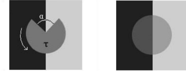
Figure 5: Illustration of the episcotister model of transparency. When the rotation of an episcotister with a reflectance \tau and open area \alpha is fast enough (left), the episcotister introduce an impression of transparency (right).
