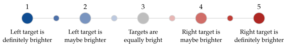
Figure 3.1: Internal coding of the rating scale. From left to right, the response categories were assigned numerical values between 1 and 5. As a result of taking the median of an even number of observations, four additional points with the values 1.5, 2.5, 3.5 and 4.5 have to be considered. These are indicated by the small, unlabeled circles.
