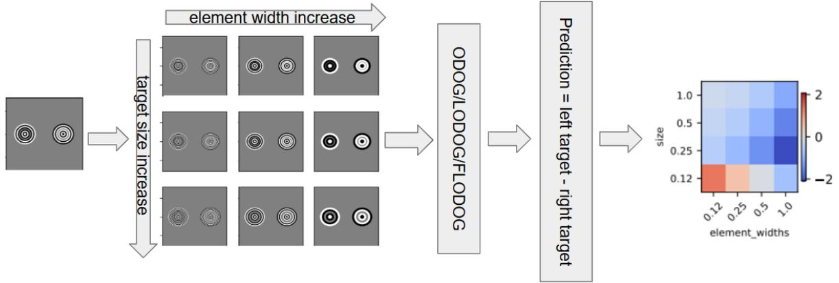
Figure 6: Workflow: First, selection of the stimuli from the Kobayashi and Shapiro (2024) research. Next, parametric variations of this stimulus are created, altering the features spatial frequency or target size. These varied stimuli are then processed by the ODOG, LODOG, and FLODOG models (middle-right), producing model outputs. From these outputs, the predicted brightness values in the target areas are extracted, calculated and assembled into a heatmap (right).
