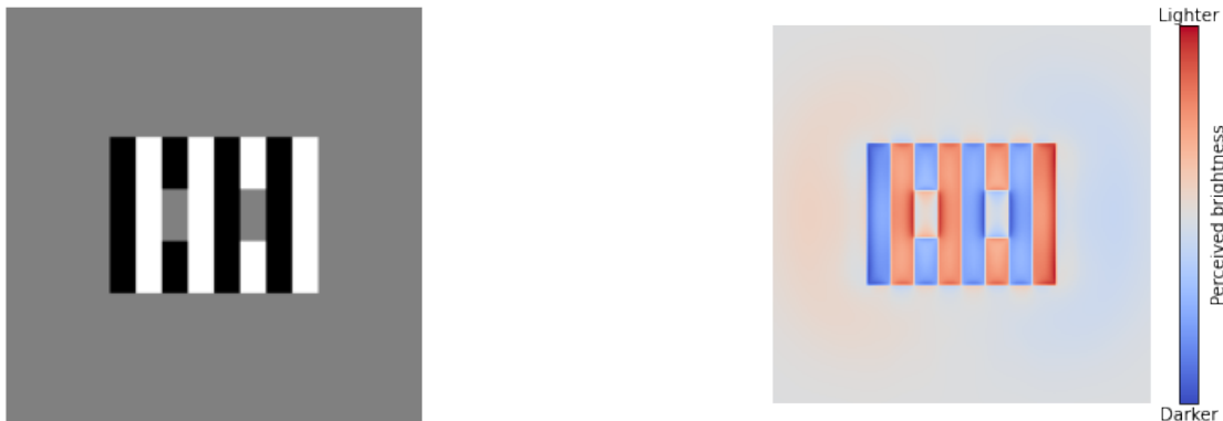
(a) Brightness perception effect, named White's-Effect[4]. The luminance of the gray patches is identical. The patch that shares more edges with the white stripes appears brighter.
