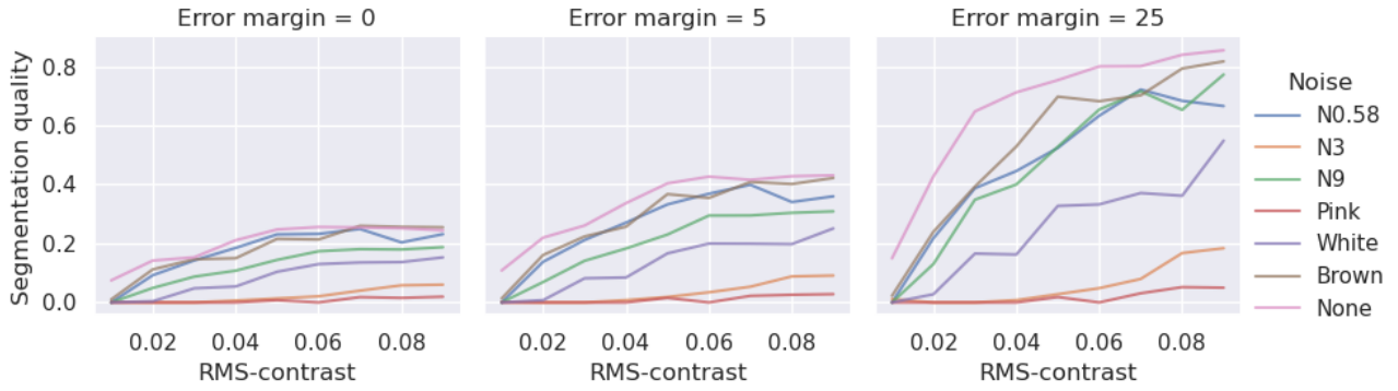
Figure 10: Results of the segmentation quality measure over the contrasts for each noise type, with the Grigorescu et al. (2003) ground truth. Each column uses a different error margin.
