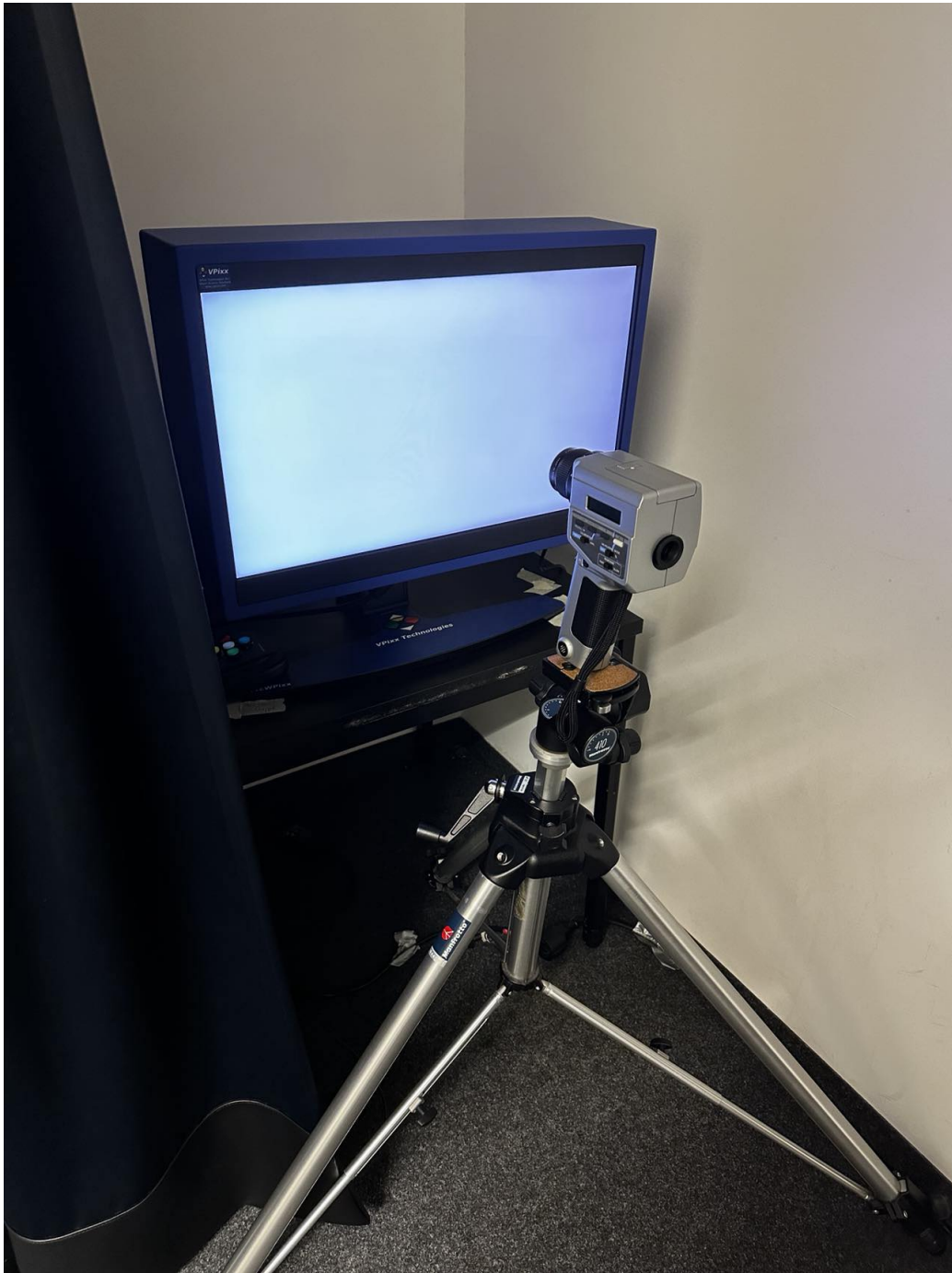
Figure 6: Measurement setup, where the photometer is aligned to the center of the monitor
